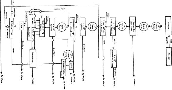
Fig. 1 .-- Flowsheet at the jig plant, Rayfield, Nigeria
