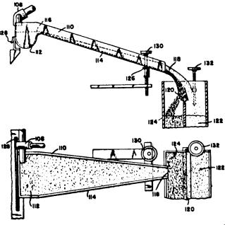
AT ROUGHER stage, the only adjustments are two screw and handwheels that tilt the sluice (132) or pliable plate (130).
