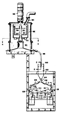
AFTER entering unit, the slurry hits a baffle and is spun to the lower vessels.
