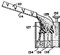
SCREW and handwheels also control the finer separation into three grades.
